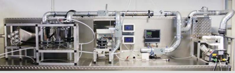
We focus on treatment effectivity, filter lifetime and total operation cost over time. The treatment methods are mainly combinations of ozone, UV and filter material. Other parameters highly affecting the tests and the final treatment solution are moisture level and concentration and type of of pollutants in the air.
