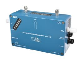
The ozone-in-water sensor BMT 964 AQ is a UV photometer for direct measurement of the ozone content of ultra-pure water, or water with constant turbidity. A special version BMT 964 AQ/HF for up to 20% hydrofluoric acid, is available. The instrument is based upon our ozone analyzer BMT 964 for gaseous ozone.
