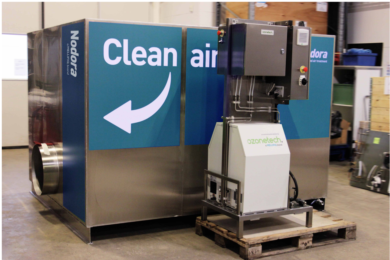
RENA Pro G-series Ozone System (front) and Nodora X3000 Activated Carbon Filter (back) ready before shipment.
